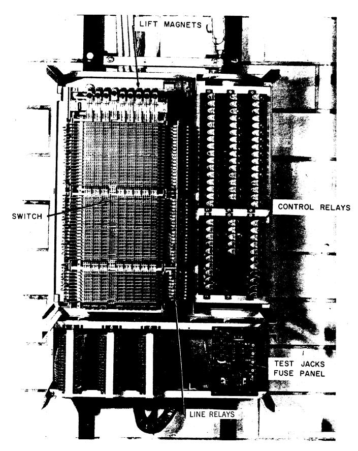
Fig. 2 – Gfeller Line Concentrator 49-9-2 Central Office Unit (Covers Removed)
