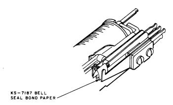
Fig. 41—Insulating Contacts of 221- and Similar-Type Relays
