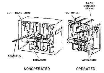
Fig. 5—Blocking C-Type Relays
