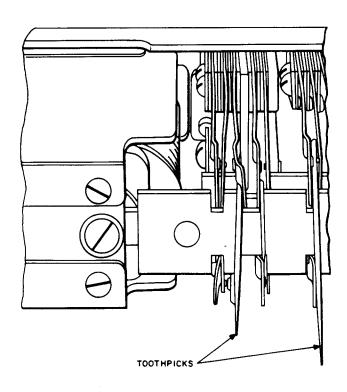
Fig. 48—Blocking Contacts of 229- and Similar-Type Relays
