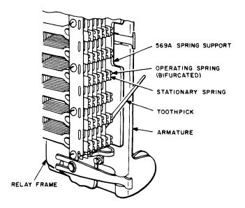
Fig. 51—Method of Blocking Individual Contacts
