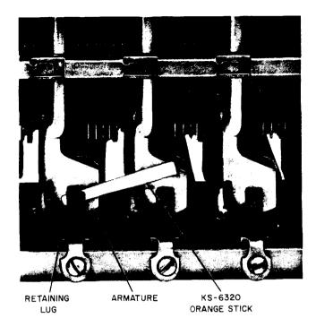
Fig 32—Blocking 324-, 325-, 328-, and 338-Type Switch Holding Magnets - Operated
