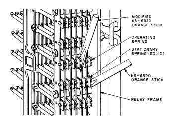
Fig. 50—Method of Blocking Individual Contacts on 263- and Similar-Type Relays
