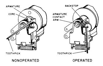
Fig. 21—Blocking 208- and 214-Type Relays
