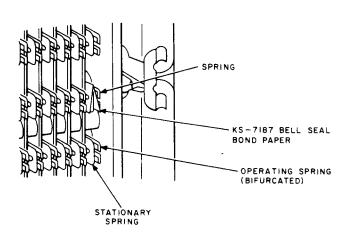
Fig. 42—Insulating Contacts of 245- and Similar-Type Relays
