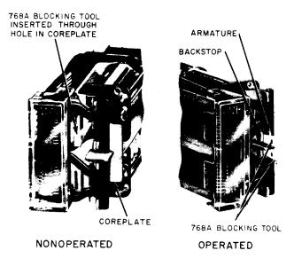
Fig. 9—Blocking AK- and AM-Type Relays
