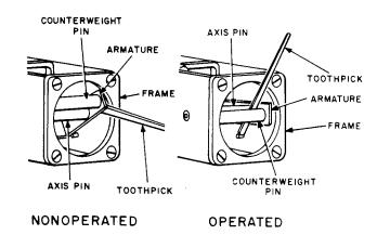
Fig. 18—Blocking 186-Type Relays
