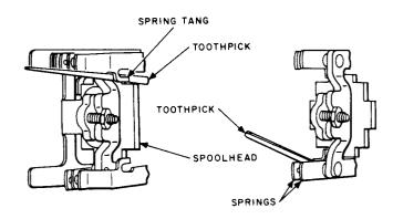
Fig. 46—Blocking Contacts of E- and Similar-Type
