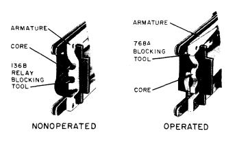
Fig. 3—Blocking Operated and Nonoperated EA-Type
