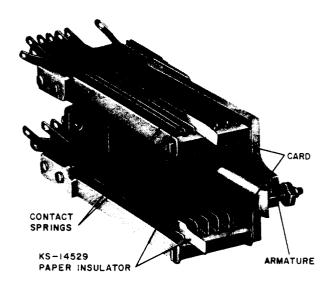
Fig. 45—Insulating Contacts of UB-Type Relays
