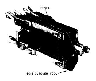
Fig. 38—Blocking U676 and U680 Relays for Cutover Purposes
