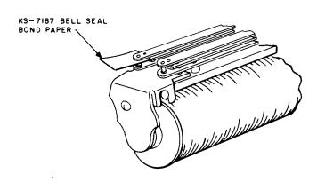
Fig. 43—Insulating Contacts of Stromburg-Carlson 200-Type Relays
