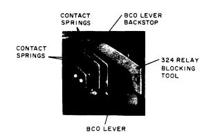
Fig. 28—Blocking Plunger-Type Line Switches - Operated
