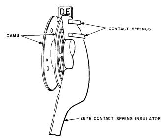
Fig. 52—Method of Using 267B Contact Insulator
