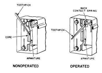
Fig. 4—Blocking B-, G-, and J-Type Relays
