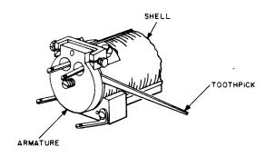
Fig. 13—Blocking 44-Type Relays - Nonoperated
