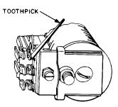
Fig. 47—Blocking Contacts of 125- and Similar-Type Relays
