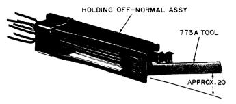
Fig. 33—Method of Blocking Holding Off-Normal Assembly
