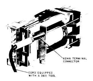
Fig. 10—Connecting to Winding Terminal of the AF-, AG-, AJ-, and AL-Type Relays (Wire Spring)
