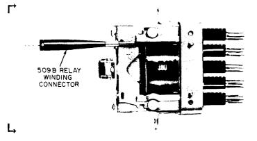
Fig. 12—Connecting to Winding Terminal at 286-, 287-, or 288-Type Wire Spring Multicontact Relay (286-Type Shown)
