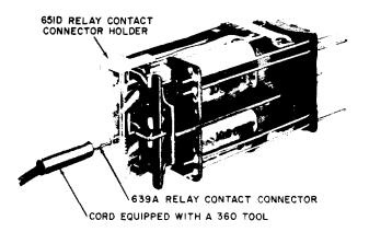
→ Fig. 16—Connecting to Fixed Contact of the AK- or AM-Type Relays (Wire Spring)
