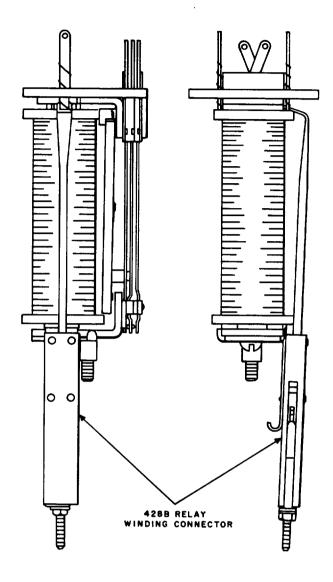
Fig. 4—Connecting to Winding Terminal of a 149-Type Relay
