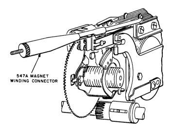
Fig. 5—Connecting to Winding Terminal of a 1-Type Timer
