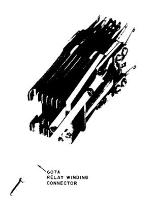
Fig. 3—Connecting to Winding Terminal of a U-Type Relay
