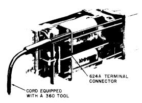
Fig. 11—Connecting to Winding Terminal of the AKor AM-Type Relays (Wire Spring)
