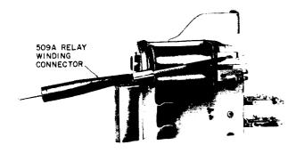
Fig. 9—Connecting to Winding Terminal of a 263-Type Multicontact Relay
