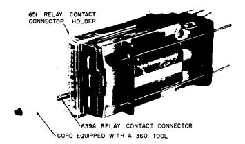
Fig. 15—Connecting to Fixed Contact of the AF-, AG-, AJ-, or AL-Type Relays (Wire Spring)
