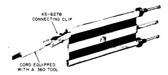
Fig. 13—Connecting to Ferrule of the 18- and 19-Type Resistors
