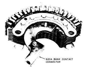
Fig. 14—Connecting to Terminal of the Step-by-Step Line Finder Switch Bank
