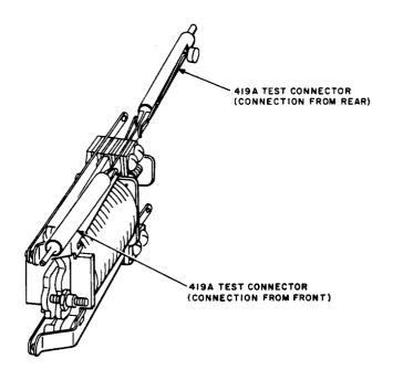
Fig. 1—Connecting to Winding Terminal and Spring of an R-Type Relay
