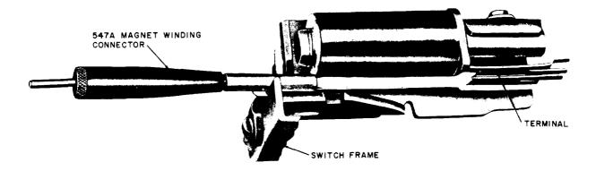
Fig. 8—Connecting to Winding Terminal of the Hold Magnet of the 324-, 325-, 328-, 334-, and 338-Type Switches
