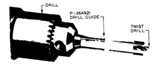
Fig. 1 - Mounting Drill Guide and Drill for Removing Rivets
