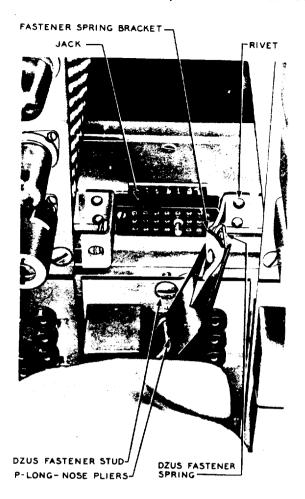
Fig. 3 - Method of Bending Bracket to Gain Access to Rivet
