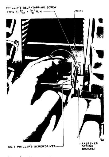
Fig. 6 - Method of Guiding Screws Into Place
