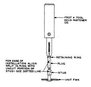
Fig. 7 - Method of Mounting Stud
