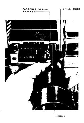
Fig. 4 - Method of Removing Rivet Heads Using Drill Guide
