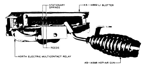
Fig. 3 - Removing Contact Protectant
