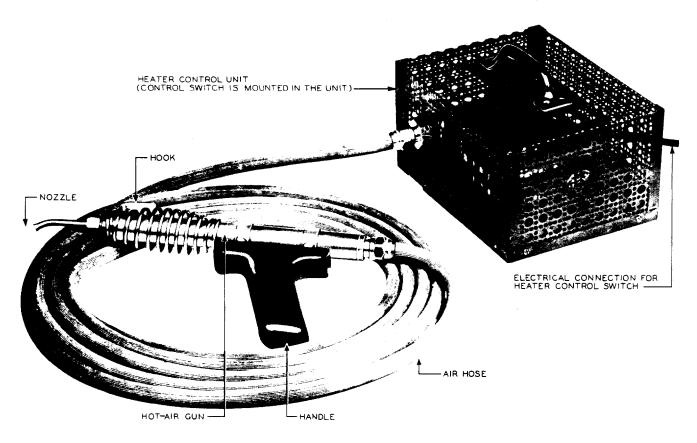
Fig. 2 — KS-14586 Hot-air Gun (Consisting of Hot-air Gun, Heater Control Unit, and Air Hose)
