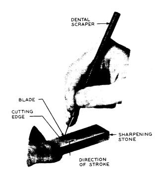
Fig. 3 - Sharpening of Dental Scraper
