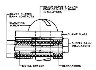
Fig. 1 - Partial Section of Bank Showing Relation of Parts
