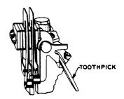
Fig. 2 - Method of Blocking Vertical Off-normal Springs in Their Unoperated Position
