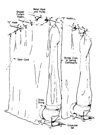
Fig. 4—Curtains With Exhauster Sets in Place
