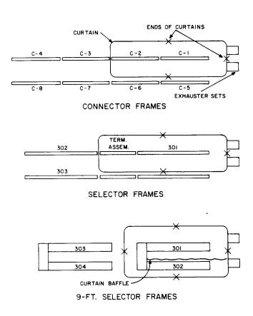
Fig. 2—Curtains in Place Around Equipment Frames to be Cleaned
