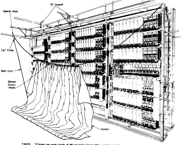
\* NOTE: "S"Hooks are made locally of #6 Insulated Copper Wire, used to support Sash Cord when in place.
