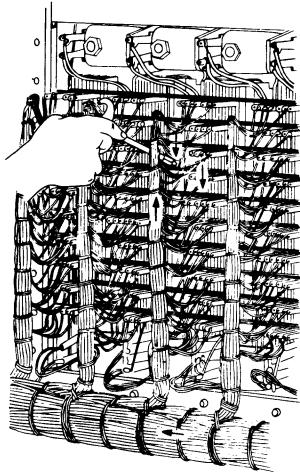
First operation downward to left or right of vertical form to remove dirt from wires and wiring lugs.
