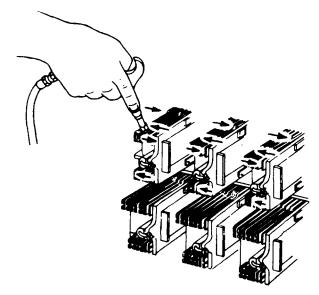
First operation to remove dirt where springs enter pile up. Second operation to remove dirt from relay coil. Third operation to remove dirt from upper contacts. Fourth operation to remove dirt from lower contacts.
