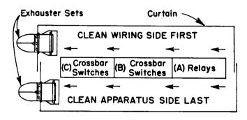
Fig. 1—Curtain Enclosed Frame With Exhauster Sets in Place
