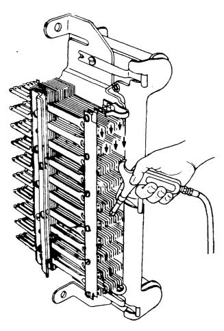
Each operation shall be downward to remove dirt from contacts and where springs enter pile up.
