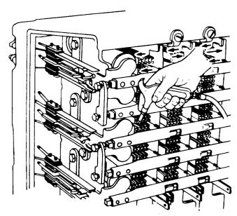
First operation to remove dirt where springs enter pile up and to remove dirt from select magnet coils.
