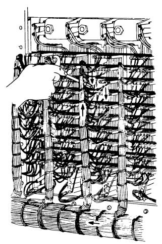
First operation downward to left or right of vertical form to remove dirt from wires and wiring lugs.
