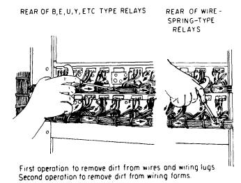
Fig. 4—Method of <u>Pireuting Nozzle for Cleaning Rear</u> of B-, E-, U-, Y-, etc, and Wire-Spring Type Relays
