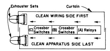
Fig. 1—Curtain Enclosed Frame With Exhauster Sets in Place
