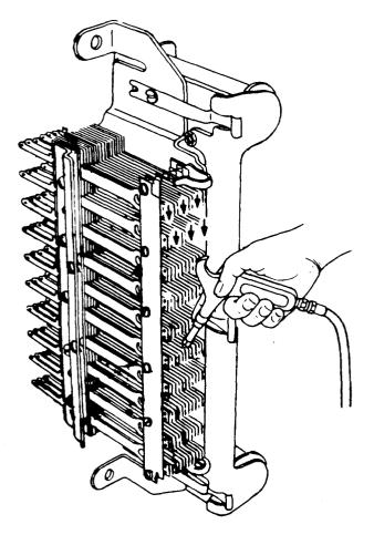
Each operation shall be downward to remove dirt from contacts and where springs enter pile up.
