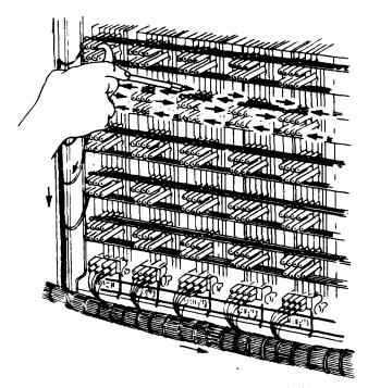
First operation to remove dirt from vertical forms and wiring. Second operation to remove dirt where wiring lugs enter spring pile up. Third operation to remove dirt where multiple strapping is soldered to wiring lugs.
