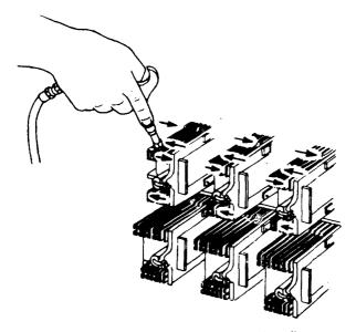
First operation to remove dirt where springs enter pile up. Second operation to remove dirt from relay coil. Third operation to remove dirt from upper contacts. Fourth operation to remove dirt from lower contacts.
