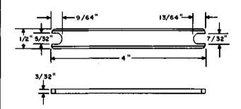
5/32- and 7/32-inch open double-end flat wrench. Replaces the 75 tool. For general use.
