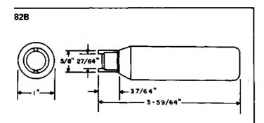
Pin wrench. Replaces the 82 tool. For use on 223-type keys.
