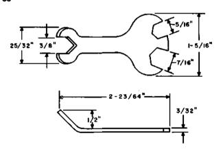
5/16-, 3/8-, and 7/16-inch hex. open-end wrench. For use on General Electric Company voltage regulators.
