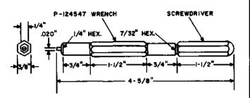
Combination 7/32- and 1/4-inch hex. double-end socket wrench and screwdriver. For general use.
