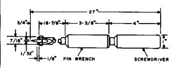
Combination pin wrench and screwdriver. Replaces the 22 tool. For use on jack fasteners.
