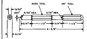
Combination 5/32- and 3/16-inch hex. double-end socket wrench and screwdriver. This tool is a combination of the 147 and 403A tools. For use on 223-type keys, spring-driven sequence switches, and relays.
