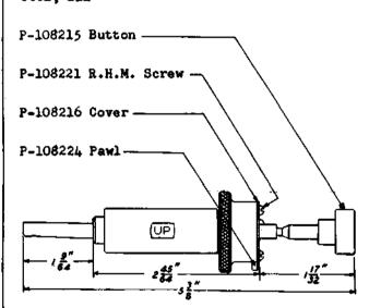
Jack spring cleaner. This tool has a roughened steel ribbon which can be inserted between the jack contacts without crossing the springs or sleeve.
