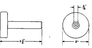
5/16-inch hex. single-end socket wrench. For use on 214A selectors of 1-type translators in 4A Toll System.
