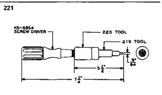
Consists of 3/16-inch and 5/16-inch hex. single-end socket wrenches and a screwdriver. This tool is a combination of the 219 and 220 tools and the KS-6854 screwdriver. For use on flat-type relays.
