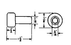
5/16-inch hex. single-end socket wrench. This tool forms part of the 221 tool. For use on 51-type dial testers.
