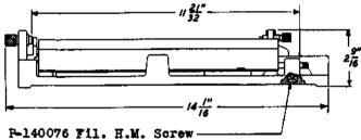
Cam aligning fixture. Consists of a metal base with fixtures for mounting a sequence switch cam shaft assembly. Provided with a straightedge for marking and realigning the cams and clamp to hold the cam shaft assembly rigid.
