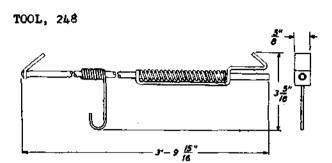
Portable lamp fixture. An adjustable support arranged to attach to channels or angles of panel type frames. Adjustable for different width frames.
