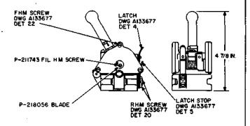
Cord cutter. The base is provided with screw holes for attaching to the KS-5263 cord repair table. For use in repairing switchboard cords by the punched hole method. The information covered herein replaces the part of Section 074-000-006, Issue 1, applying to this tool.
