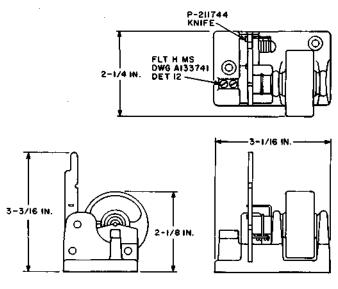
Conductor braid cutter. For use in repairing switchboard cords by the punched hole method. The information covered herein replaces the part of Section 074-000-006, Issue 1, applying to this tool.
