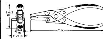
Brush spring crimper. For use on 14-type commutator brushes.
