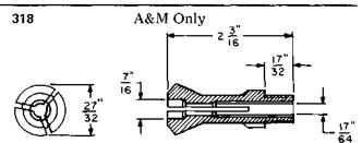
Plug remover and attacher. This tool, in conjunction with the 200 tool, is equivalent to the 317 tool. Do not order this tool unless the office is equipped with the 200 tool.
