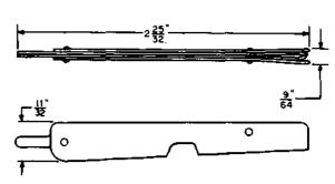
Spring contact clip and insulator. Replaces the 250 tool. For use on A- and B-type sequence switches and panel elevator apparatus.
