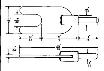
Spade terminal. For use in conjunction with a 360-type tool for general test purposes.
