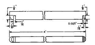
Adjuster. For use on E1- and E2-type keys.
