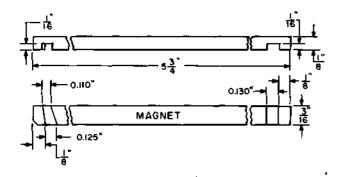
Adjuster. For use on E1- and E2-type keys.
