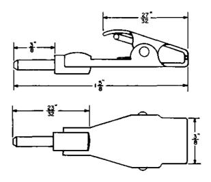
Connecting clip. For use in conjunction with a 360-type tool for general test purposes.
