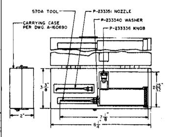
Oil gun. Designed to discharge oil in definite limited quantities. Furnished with a wooden carrying case and two nozzles, one straight and one curved.
