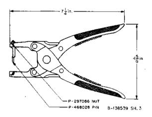
Pawl Pin Remover. This tool forms part of the No. 1001A tool kit.
