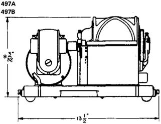
Plug Cleaners. The No. 497A tool is for a-c operation. The No. 497B tool is for d-c operation.
