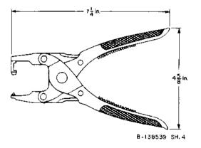
Pawl Pin Replacer. This tool forms part of the No. 1001A tool kit.
