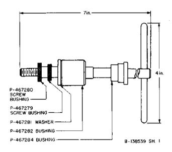
Bushing Remover and Replacer. This tool forms part of the No. 1000A tool kit.
