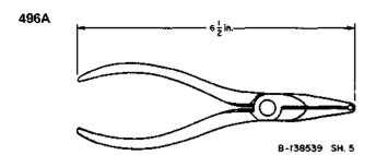
Pin Pliers. This tool forms part of the No. 1001A tool kit.
