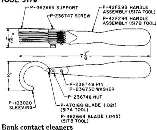
The blades and support of the 402E tool may be used in the handle of the 517A tool.
