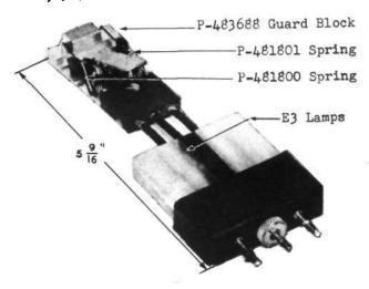
Contact Closure Indicator. This tool forms part of the J94724 contact closure test set.
