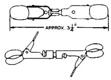
Cord Support. This tool forms part of the J94724 contact closure test set.
