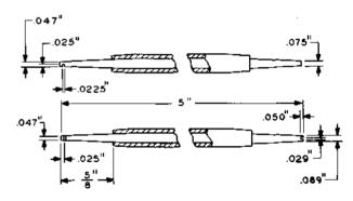
Contact aligning tool
