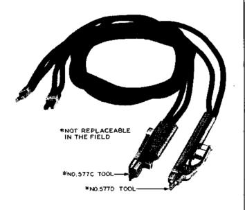
Welding pliers equipped with 57" leads
