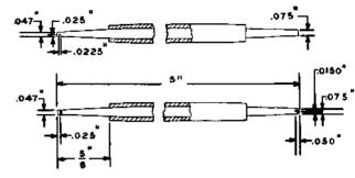
Contact aligning tool
