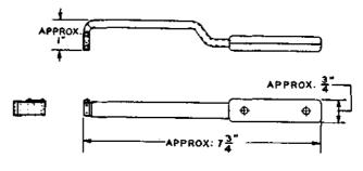
Commutator brush guide mounting tool
