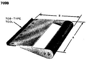
Handle (shown with 708-type tools forming comb for removing contact protectant compound.)
