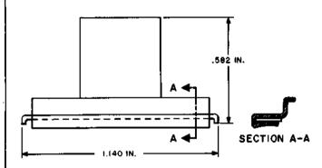
Insulator. For use in insulating levels 1 through 9 of the 9A commutator of step-by-step switches in No. 1, 350, and 355A step-by-step central offices during test procedures.
