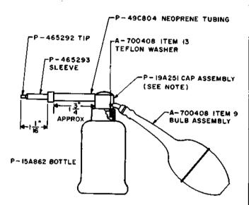
Note: When ordering the P-19A251 cap assembly, also order one A-700408 Item 13 Teflon washer. Thread washer on cap before mounting cap on bottle.
