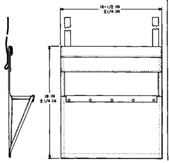
The KS-20962 L1 connecting bag is used in collecting small pieces of wire and solder drippings while working on apparatus such as main distributing frames. The bag is rubber lined and is made of a flame proof cotton duck material. It is 9-1/4 inches high by 16-1/2 inches wide and has a 4-inch wide opening with a weighted flap, two side pockets, and two straps for securing the bag to the frame.
