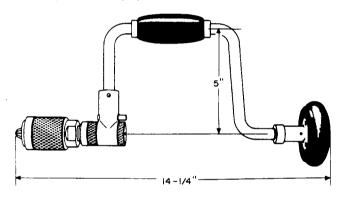
Jaws take square bit stocks up to 5/8-inch across corners and straight or tapered shanks up to 1/2-inch in diameter. Replacement parts listed below may be ordered:
