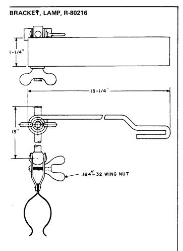
Designed to hook over the top angle of step-by-step switch shelves. The bracket has an adjustable arm for holding a portable lamp guard in various positions. For use in checking and adjusting step-by-step switches and associated apparatus.
