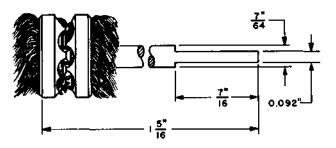
Replaces but not interchangeable with the 133 tool (spring cleaning tool). For use in conjunction with 1495 WE all-angle drill.
