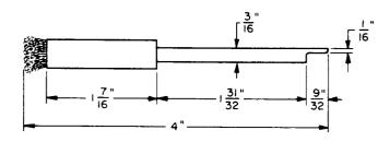
Order this tool for replacement purposes only. Replaced by, but not interchangeable with, the KS-6916 wire brush.
