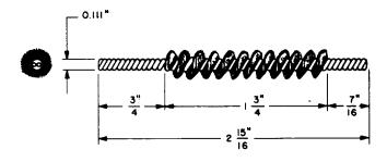
A soft nylon bristle brush. Replaces the R-2448 treating brush. For cleaning sequence switches and panel multiple banks.
