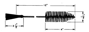
A bottle-type typewriter brush having a twisted wire handle 12 inches long. For use on friction roll drives and plunger-primary and secondary line and out-trunk switches.
