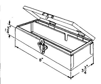
A metal case finished in olive green enamel. For housing and carrying tools and gauges for adjusting apparatus in the Crossbar System.
