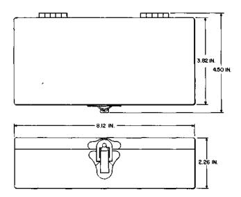
A rectangular-shaped metal container equipped with a hinged cover and latch. This case is part of the KS-20558 L1 tool kit. See Section 074-232-112.
