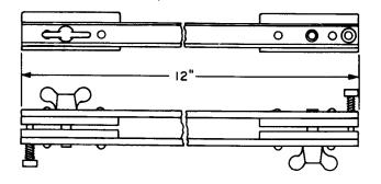
Fig. 1-585A Clamping Tool
