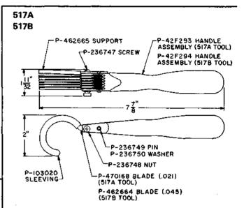
Bank contact cleaners. The blades and support of the 402E tool may be used in the handle of the 517A tool. The 517A tool replaces the 402D tool and is used in cleaning the contacts of 200-point banks of 197-type switches.
