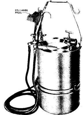
Mounts three KS-14686 pads which are arranged to scrub six cam sides simultaneously. The pads must be ordered separately. Refer to Section 069-601-801 for piece-part data and maintenance information for this tool. Replaces the 435A tool. For use in cleaning cams of sequence switches and 157-type interrupters.
