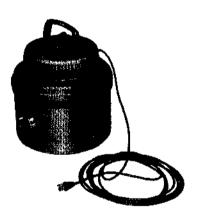
Portable upright tank-type vacuum cleaner for use where heavy duty or silent type, such as KS-14377, is not required. It is approximately 11 inches in diameter and 13 inches high, exclusive of handle. Weight, without attachments, is approximately 17 pounds. It may be mounted on a rolling ladder by using a 32B ladder bracket. It is equipped with a three-wire 19-foot long KS-14410 L31 power cord. For general use.
