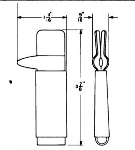
Cushion placing clip. Used in conjunction with 515A tool. For placing 1A and 2A cushions on 109, 309, 110, or 310 plugs. Also for placing 4A cushions on 47- or 347-type plugs. Replaces the KS-7872 pliers.
