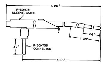
Fig. 15-770B Test Connector Tool
