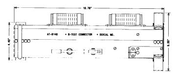
Fig. 16-AT-8148B Test Connector Tool
