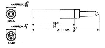
Fig. 12—624A or B Terminal Connector Tool
