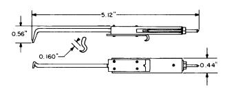
Fig. 4—428B Relay Winding Connector Tool
