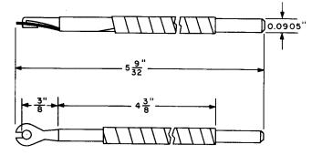
Fig. 10-607A Relay Winding Connector Tool
