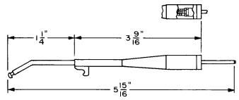
Fig. 9—548A Magnet Winding Connector Tool
