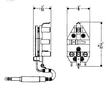
Cord shelf connecting tool. Furnished with a W3N cord and a 110 plug. Replaces the D-87336 tool. For use in making connections to cord circuits in local and toll switchboards.
