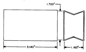
For use with the B-1185 relays having potential on frame as in disabler circuits associated with E2 and E3 repeaters.
