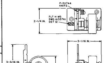
Conductor braid cutter. For use in repairing switchboard cords by the punched-hole method. The information covered herein replaces the part of Section 074-000-006, Issue 1, applying to this tool.
