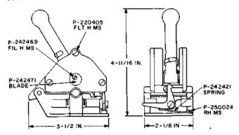
Cord cutter. The base is provided with screw holes for attaching to the KS-5263 cord repair table. For use in repairing switchboard cords by the solderless cord-tip method.
