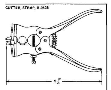
For cutting slots in straps to separate groups, when required, on 15-type banks.
