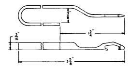
Tab depressor. For checking spring pressure on 304-, 324- and similar-type switches.
