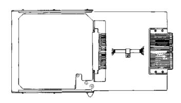
The extender was developed for use with the 4A toll miniature wire spring relay trunk circuits to provide access to the circuit boards. The extender will plug into any position of any housing on the frame.
