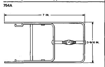
Extractor tool. For use in removing KS-19162 L14 plugs used on interconnecting switchboard cables between two No. 5 crossbar completing marker frames.
