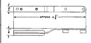
Extractor tool. For use in removing E2 and E3 telephone repeaters from mounting shelf.
