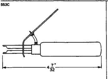
Lamp extractor. For use in removing No. 2 telegraph service board lamps.
