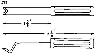
Signal plug extractor. For use in extracting signal plugs from multiple jacks and 350A make-busy plugs at outgoing trunk test frame.
