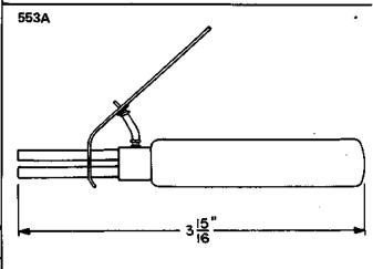
Lamp extractor. Replaces the 116 tool. For use in removing switchboard lamps.
