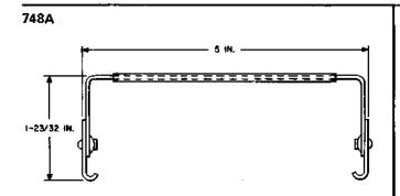
Extractor tool. Was intended initially for use in extracting printed wiring board circuit packs of a data set in the No. 1 Electronic Switching System.
