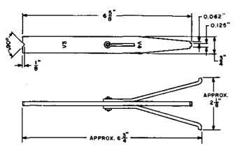
Amplifier extractor. Replaced the 602C tool. For use in removing the plug-in amplifiers associated with V3 and V4 repeaters from their shelf mountings.
