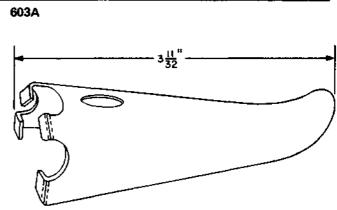
Relay extractor. For use on 275-, 276-, 291- and 303-type relays.
