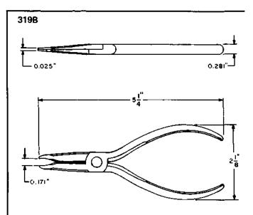
Lamp cap and number plate extractor. Replaces the 87, 112, 125, 146 and 319 tools. For use in removing 2-, 4-, and 8-type lamp caps and 59-, 60- and similar-type number plates.
