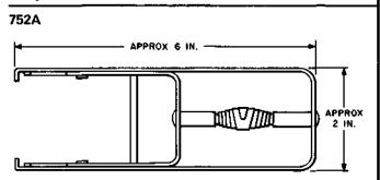
Circuit pack extractor. For use in removing D-type circuit packs from 910-type connectors.
