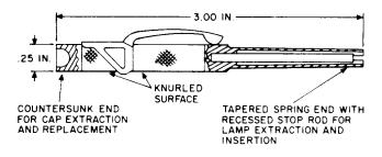
Fig. 12—KS-21144, L1, Lamp and Cap Extractor
