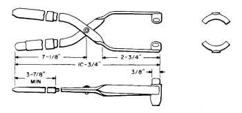
Fig. 5—KS-5637, L1, Tube Extractor
