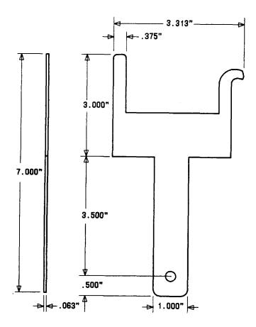
₱Fig. 3—811A Printed Wiring Board Extractor
