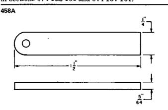
Indicator finger. Replaces finger of bracket and finger R-2166. For use with the 121A gauge on reciprocating bar-type interrupters.
