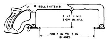
The B hacksaw frame accommodates 8-inch to 12-inch hacksaw blades. Blades for hacksaw frame must be ordered separately. See Blades, Hacksaw, for lengths and teeth per inch. For general use.
