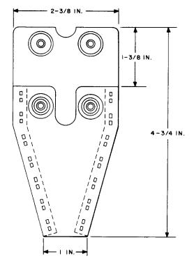
Replaces shave hook guard AT-6893. For use on B shave hook AT-7151. (Specification AT-7151)
