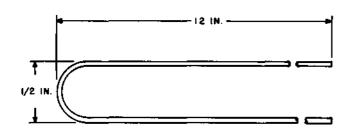
Hairpin guide. Used as an aid for replacing defective hairpin select wires with the vertical units of a small crossbar switch mounted in an equipment frame.
