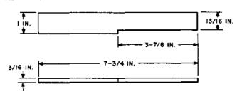
For use in replacing worn contact springs of sequence switches.
