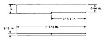
For use in replacing worn contact springs of sequence switches.
