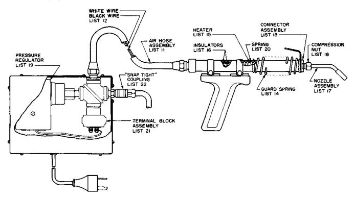
Hot-air gun. Consists essentially of a gun, an air-hose and a current control unit. Operates on 115 volts ac or dc with a power consumption of 300 watts.
